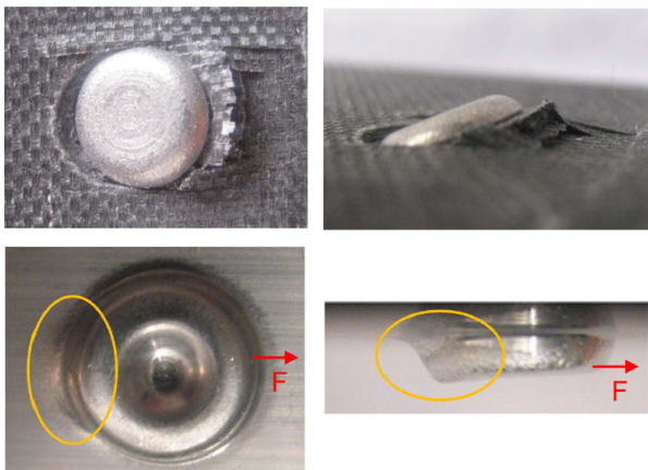
Fig. 11. Plastic deformation of the bottom aluminium alloy sheet leads to a tilting rivet and thus to a brittle damage of the upper CFRP laminate.
